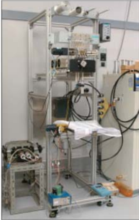
Carbon dioxide laser-thinning apparatus used for preparation of nonwoven fabric that was made of endless microfibers.
